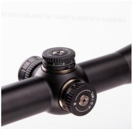
**STEP 2:** Unscrew the bolts holding the turret scales with Allen key.
